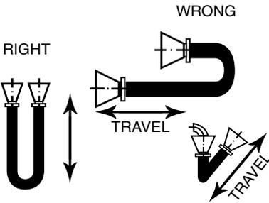
Prevent twisting, torque or distortion, hose should be bent in same plane as motion.
