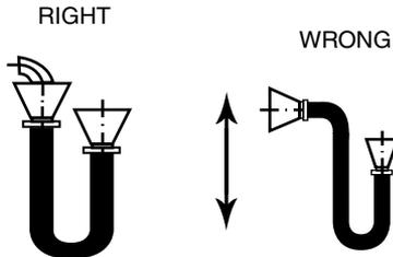
Never place sharp hose bends near coupling. Hose should be installed so that flexing takes place in one plane only & direction of motion must be perpendicular.
