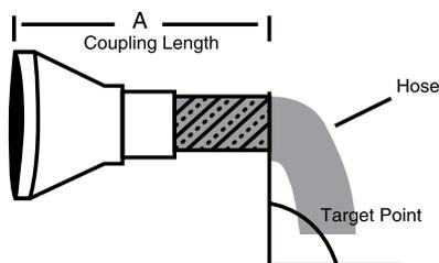
12. If there is the potential of a pull-away, buttressing of the piping system is a must. This will prevent piping fracture and make the hose the weakest link, causing it to separate. It is recommended to use a break-away device along with dry-brake couplings for those applications with hazardous chemicals that may cause human injury or environmental damage.
