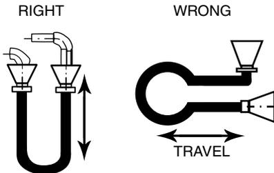
When the hose minimum bend radius is exceeded, use angled adapters to meet radius requirements.
