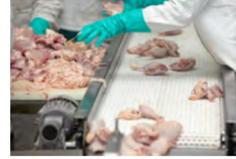
Sealed belt edges and appropriate belt splicing methods support hygienic processing.
