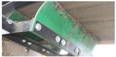
Apache's Infinity Finger Scraper is designed to act as both a primary and secondary scraper all-in-one unit, cleaning more effectively and efficiently than a traditional belt brush. Specifically designed for use on cleated, non-cleated, and textured conveyor belting, with or without mechanical fasteners, the Finger Scraper will reduce carryback from 1 to 3% – decreasing maintenance and cleanup costs.
